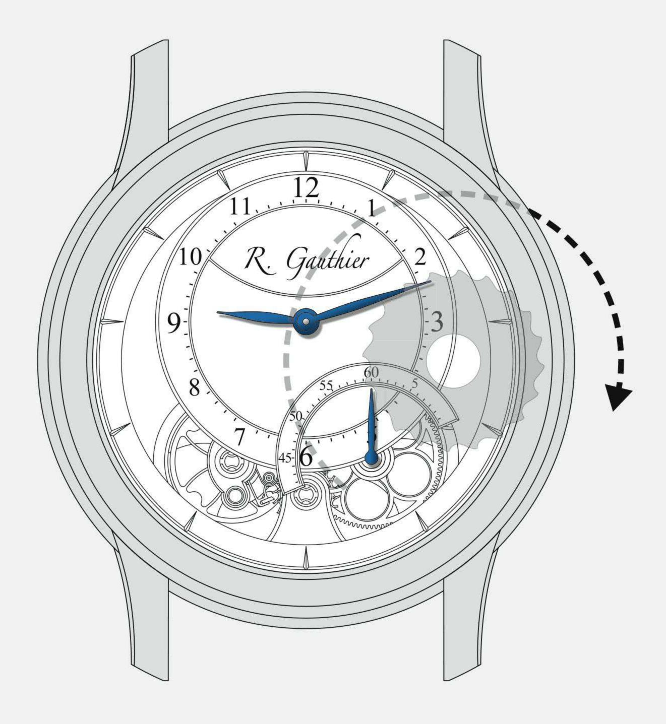
Prestige HM/HMS can also be wound while on the wrist, by placing your thumb on the caseband and using your index finger to turn the crown.
