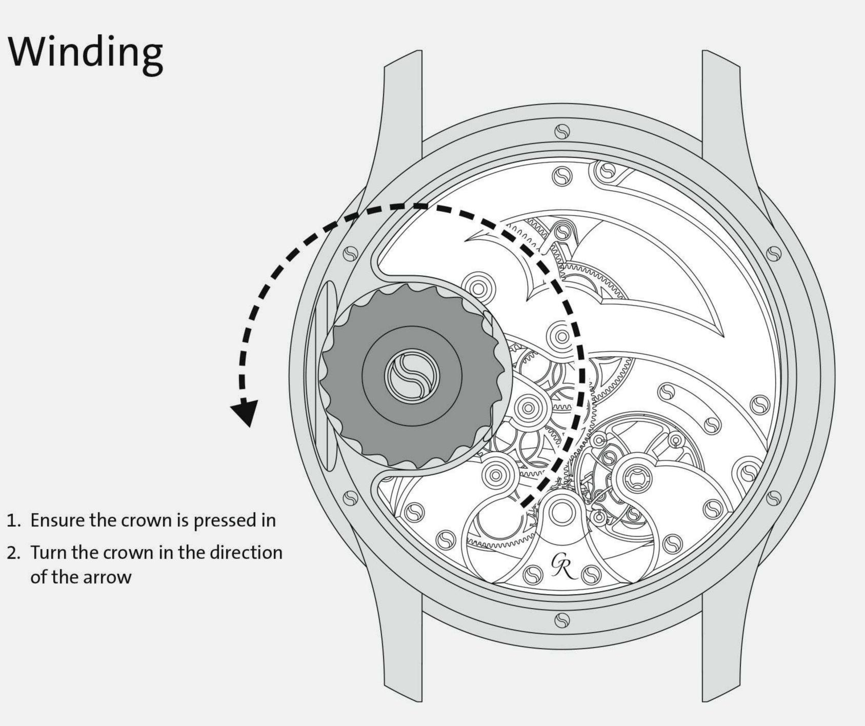
Prestige HM/HMS is manual winding timepiece. It is wound using the crown on the caseback.
