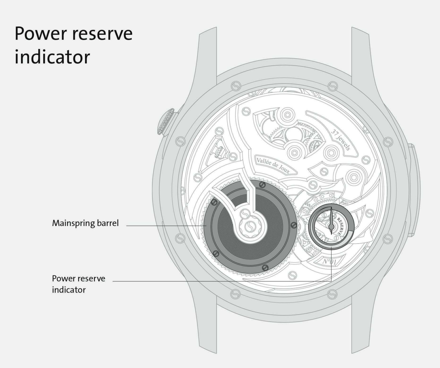
The power reserve indicator is visible on the back of the movement and shows the state of wind of the mainspring from "OFF" (no power) to "POWER ON" to "FULL" (46 hours of power reserve).
