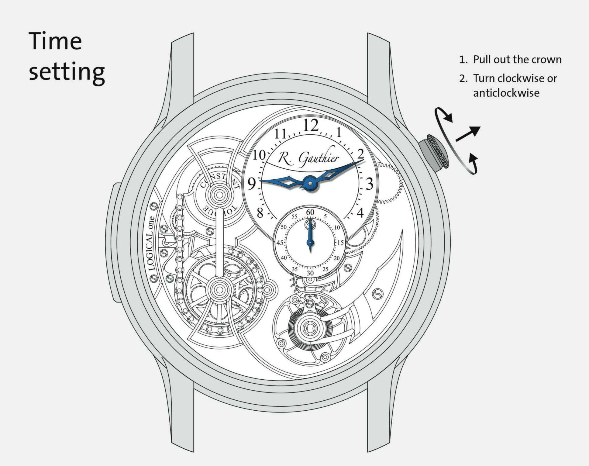
The time is set on Logical One using the small crown on the caseband at 2 o'clock.
