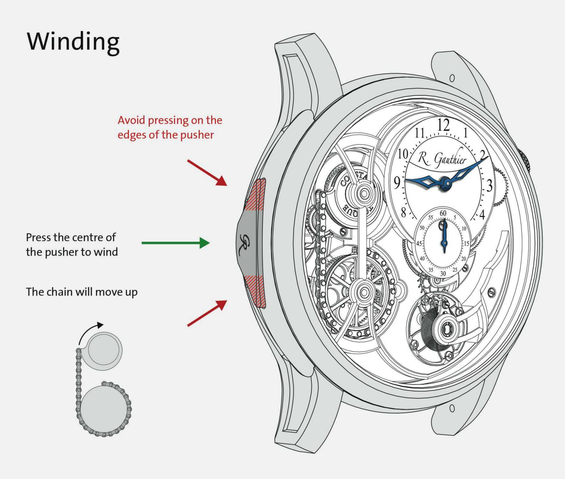
Logical One is a manual winding timepiece. To wind it, press the integrated caseband pusher fully in towards the case.
