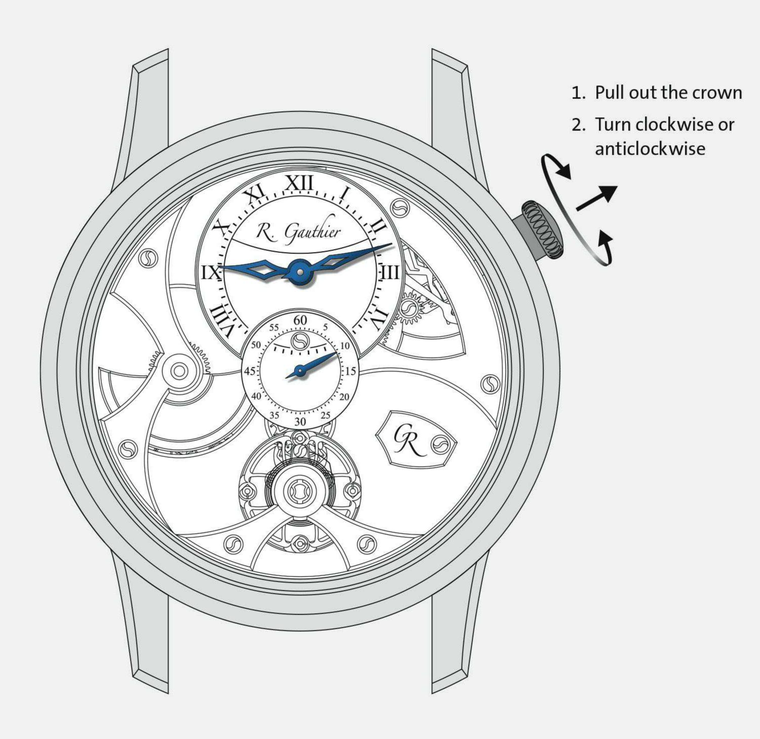
To set the time on Insight Micro-Rotor, gently pull out the crown at 2 o'clock. You should hear and feel a small click when the crown is fully out.
