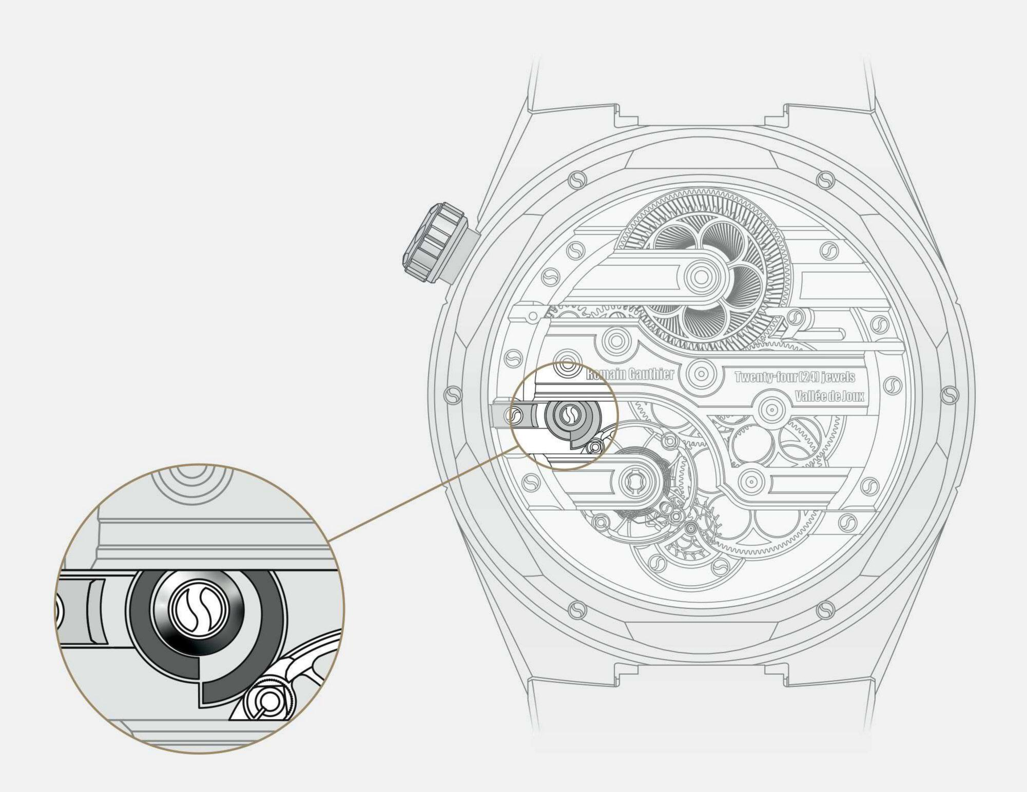
Position of the snail cam during time setting.
