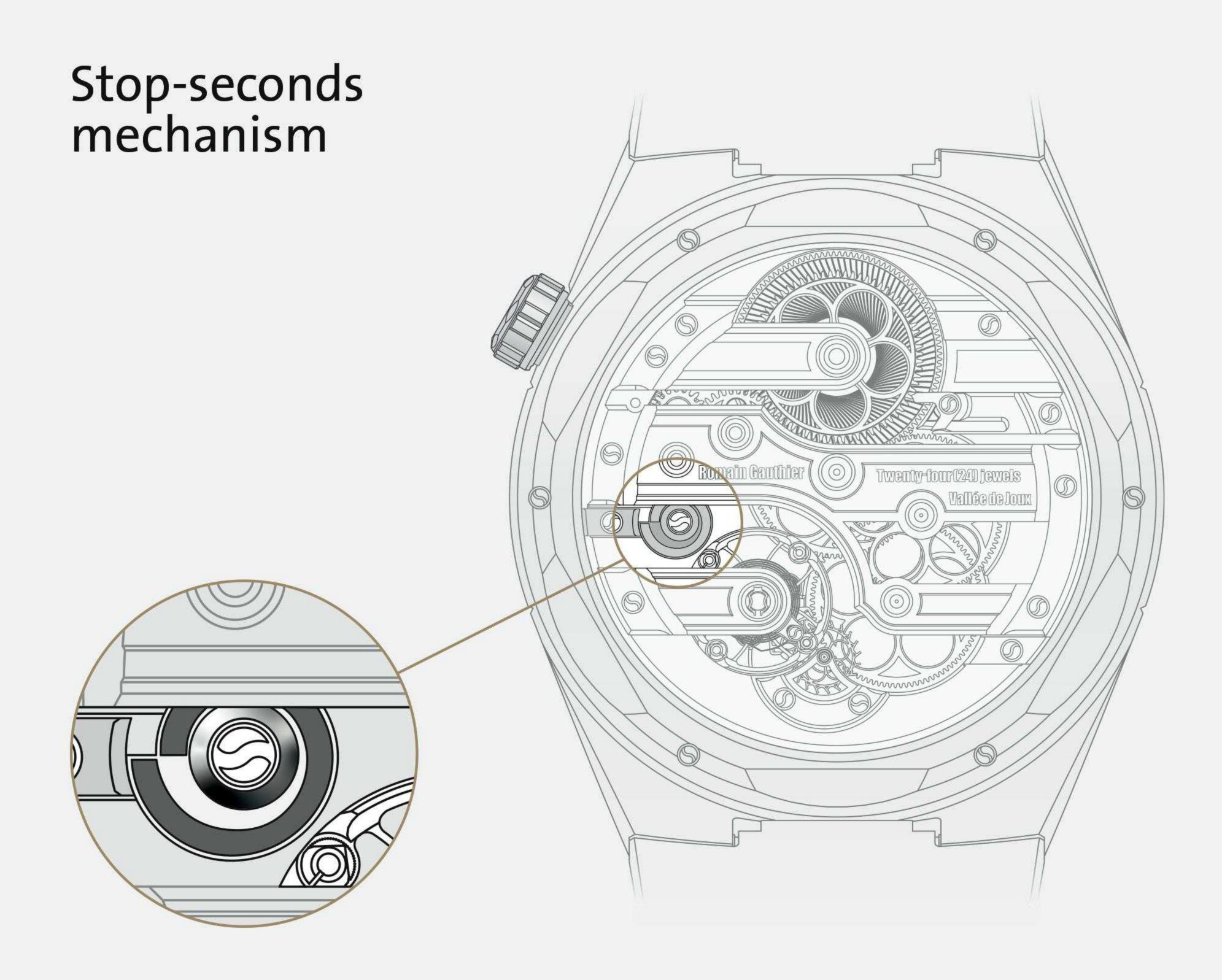
Position of the snail cam when the watch is working.
